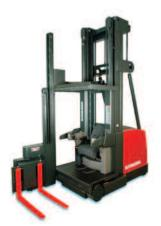
on their new 9000 Series Swing-Reach® lift truck. While the 9000 Series features energy saving technology, it also is designed to provide operators with smooth and precise motion control. This includes the movement of the truck and the movement of the mast.
