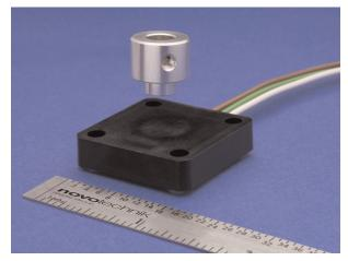
The two-part design of the RFC 4000 Series - a sensor and its magnetic position marker - offer unlimited mechanical life. The RFC Series position marker mounts on a rotary shaft, a distance from the detecting sensor component, and the magnetic field orientation is captured using an integrated circuit. An analog output signal represents the calculated angle and is repeatable to  $\pm$  1 LSB.
