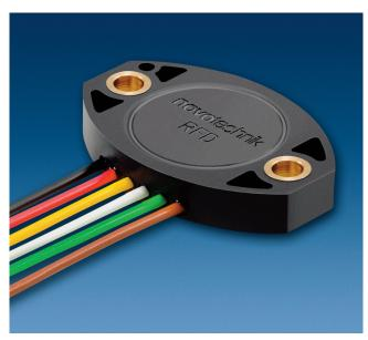
A magnetic position marker is attached to a rotating shaft or part on your application using two mounting holes. The RFD4000 Series sensor uses a Hall effect microprocessor to detect the position of the magnet and convert the angle to a voltage output.
