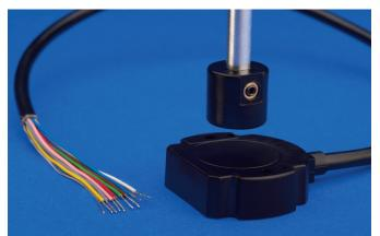
The RFC4800 Series utilizes a magnetic pickup to provide a touchless measurement range of 0 to 360°. Key specifications include ingress protection from liquids and dust to the IP 69K standard, resolution to 12 bits, repeatability of 0.1° and independent linearity of  $\pm 0.5$  %.
