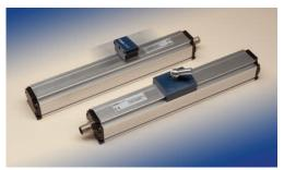
The TP1 Series is plug-in compatible with other similar sensors and is offered in standard measurement ranges of 50 to 4,500 mm. Other key specifications include update rate of 62  $\mu$ sec, absolute linearity to within ±0.02 % of F.S, 16-bit resolution and sealed to meet the IP 68 standard.
