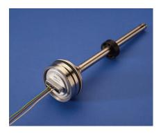
TIM sensors are easily mounted in-cylinder through one end and attached to the cylinder with either a threaded flange on the rod or a plug-in flange. Screw-plug hole is sized at M18 diameter and plug-in flange is 48 mm. A magnetic pick-up position marker is mounted on the application's piston rod.
