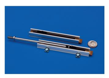
PTP Series sensors feature an ultra-compact profile of 13 mm width by 11.6 mm height. Length is dependent on the application and typically is between 10 and 300 mm. Integral guides and mounting clamps make mounting quick and other mounting options can be made.
