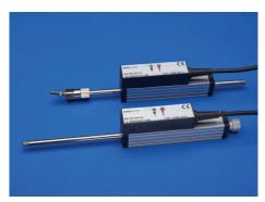
The LS1 Series feature programmable end-points using easily accessible push buttons on top of the sensor. Programming is achieved using a signal processor integrated into the sensor and two LED programming status indicators. An output range can be programmed either the same as, or independent of, actual travel length by setting minimum and maximum output levels. Current or voltage output levels can be programmed separately from position programming.
