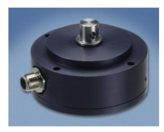
Combining stainless steel shaft and anodized aluminum housing construction with ultrahigh IP rating make the IPX salt water resistant and splash proof. The IPX Series is also designed to operate under wide temperature conditions from -40to +120 °C as well as in the presence of high– humidity dust, shock and vibration.
