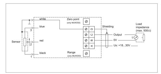
The output signal rises when the position transducer actuating rod (LWH) or actuator (TLH) is moved from 1 to 3 (status on delivery). If the reverse action is required, the terminals 1 (black) and 3 (blue) must be exchanged at the socket insert. After removing the transparent lid, the socket insert can be pushed outwards.
