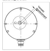
Lateral magnet offset will cause additional linearity error. The angle error, which is caused by radial displacement of sensor and position marker depends on the used position marker or magnet.
