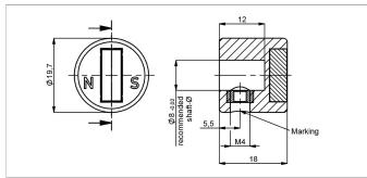
Position marker for fixation with threaded pin M4 (included in delivery)
