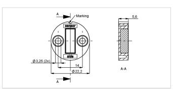
Position marker for frontal fixation with 2 cylinder
