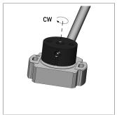
When the marking of the position marker is pointing away from the cable, the output is in the vicinity of the reference pulse (Z).
