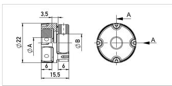
Backlash-free, double cardanic shaft coupling for Ø6 mm to Ø6 mm, Ø6.35 mm or Ø10 mm, mounting via 2 threaded pins with internal
